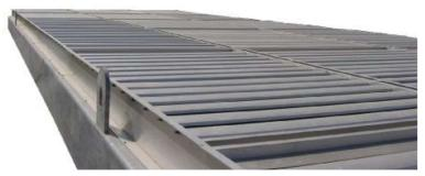
Louvers are designed both for induced and forced draft applications. For forced draft application, the louver frame is made of Aluminum sections and for induced draft the frames are made of Carbon Steel.
